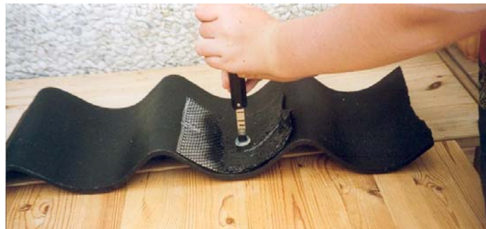
Measurement of deformation pressure and (return) springiness
