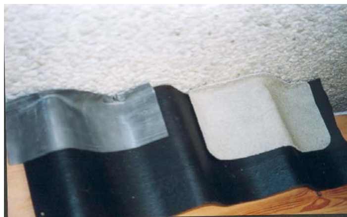
Lead and an initial sample of Perform with sand as top surface layer (September 1999)
